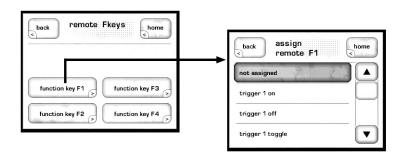
The remote control supplied with the CP-500 has four **function keys (Fkeys)** that allow you to have instant, easy access to specific system functions that might otherwise be buried in a menu somewhere.
